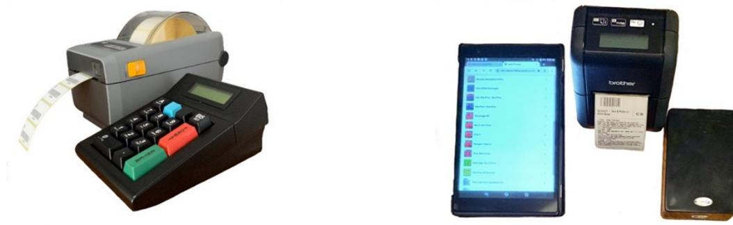
2. The 9000 PrintBox can be used with a wi-fi or wired network and a tablet computer. Most people can use a tablet computer with ease and, with a wireless network available in the shop, this configuration allows users to move the equipment around in the shop and stock room, perhaps printing the Gift Aid labels on a mobile wireless printer.
